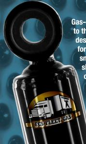
Gas-charged shocks add nitrogen to the original hydraulic shock design to enhance performance for a more responsive, smoother ride. Inside the shock, a low-pressure charge of nitrogen gas is added in the chamber above the hydraulic oil to minimize aeration of hydraulic fluid. This helps significantly reduce fade, minimize vibrations, and extend service life.
